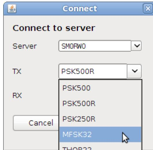
The connect buttons now open a window where you can set the TX and RX modes for the session. On a good channel you can normally leave both RX and TX modes on the default.
